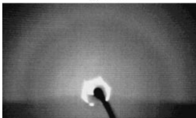
Figure 6. Top: X-ray diffraction patterns of 3a–e after heating them above the clearing point and cooling to room temperature. Bottom: X-ray diffraction pattern of an oriented sample of 3a , showing a hexagonal arrangement of the first-order diffraction peaks.
